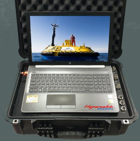
PMPT Single band mesh or Dual band mesh VHF / UHF Flight case Radio and computer for Drones & Robotics long Range Video, data & remote control.
