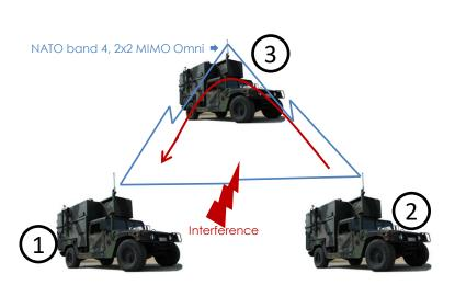
NATO band 4, 2x2 MIMO Omni NATO band 3, 2x2 MIMO Omni Hot standb Active Interference High faster change to NATO band 3 when interference
