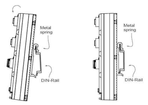
To remove the switch from the DIN-Rail, simply reverse Steps 2 and 3 above.
