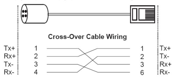
M12 (4-pin, M) to RJ45 (8-pin) Cross-Over Cable Wiring
