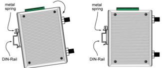
To remove the AWK-3131 from the DIN-Rail, simply reverse Steps 1 and 2.
