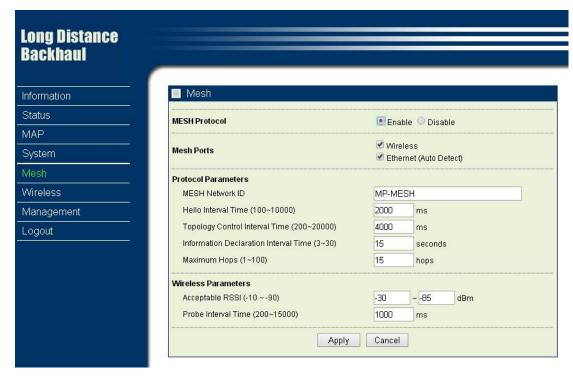
**Mesh Protocol:** You can Enable or Disable Mesh Routing protocol here.
