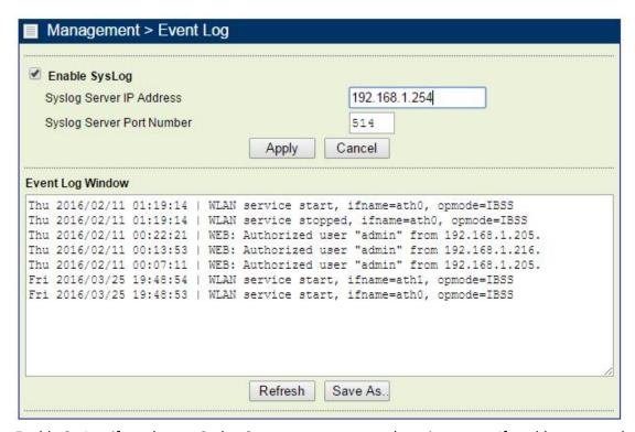
Enable SysLog if you have a Syslog Server on your network environment. If enable, you need to input the Syslog Server IP Address (default is 0.0.0.0) and the port number your Syslog Server is configured to use. The default port number is 514. The Event Log Window lists Wireless backhaul events. Click on "Refresh" to update the network events or "Save As..." to save the event into a file on your computer. Click "Apply" if you made any changes.
