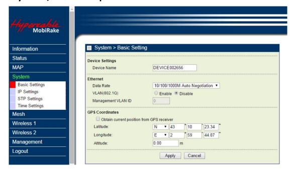
The **Device Name** is used to give a name to your 300 MHz 4x4 MIMO HT-OFDM MESH Radio. This will enable you to manage your radio more easily if there are many radios in your network.
