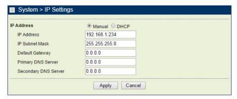
**IP Address:** Type the IP address you want to set to your 300 MHz 4x4 MIMO HT-OFDM MESH Radio (Default: 192.168.1.1).
