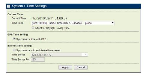
**Current Time:** While you connect this Wireless backhaul to Internet, it could automatically synchronize the current time with the Time Server that you have set.
