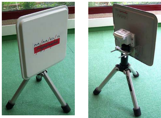
Version 3,4 - 4,2 GHz, LNB outside the antenna housing
