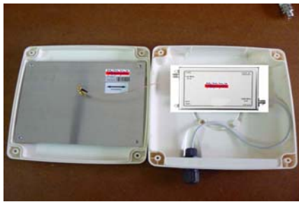
Version 4,9 - 5,9 GHz, LNB inside the antenna housing
