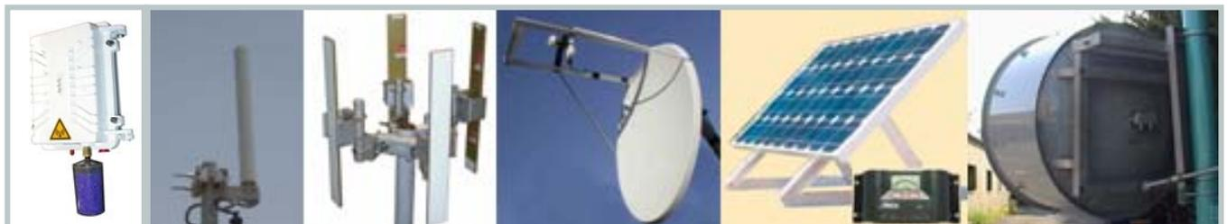
Radio TX ODU 27 dBm    Omni TX antenna 10 dB    Four sectorial TX 360° 4x17dB    High gain 90 & 120cm Inverted Gregorian 40dB    Energy by solar panels combined with wind mill    Furtive RX antenna 45- 75- 90-120-200 cm
