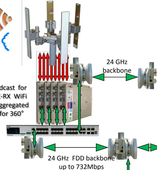
IPTV 5 GHz TX Broadcast for downstream and TX-RX WiFi
