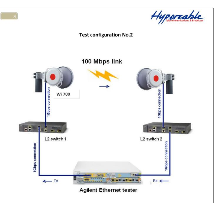
Ethernet tester's Tx port is connected to L2 switch 1 to port 1 and FODU Wi700 LAN port 2 (in WEB GUI 'LAN4') is connected to L2 switch port 2
