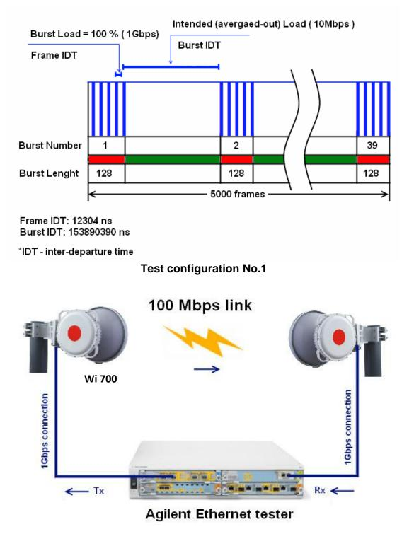
Ethernet tester's Tx port is connected to FODU WI 700 LAN port 2 (in WEB GUI 'LAN4')
